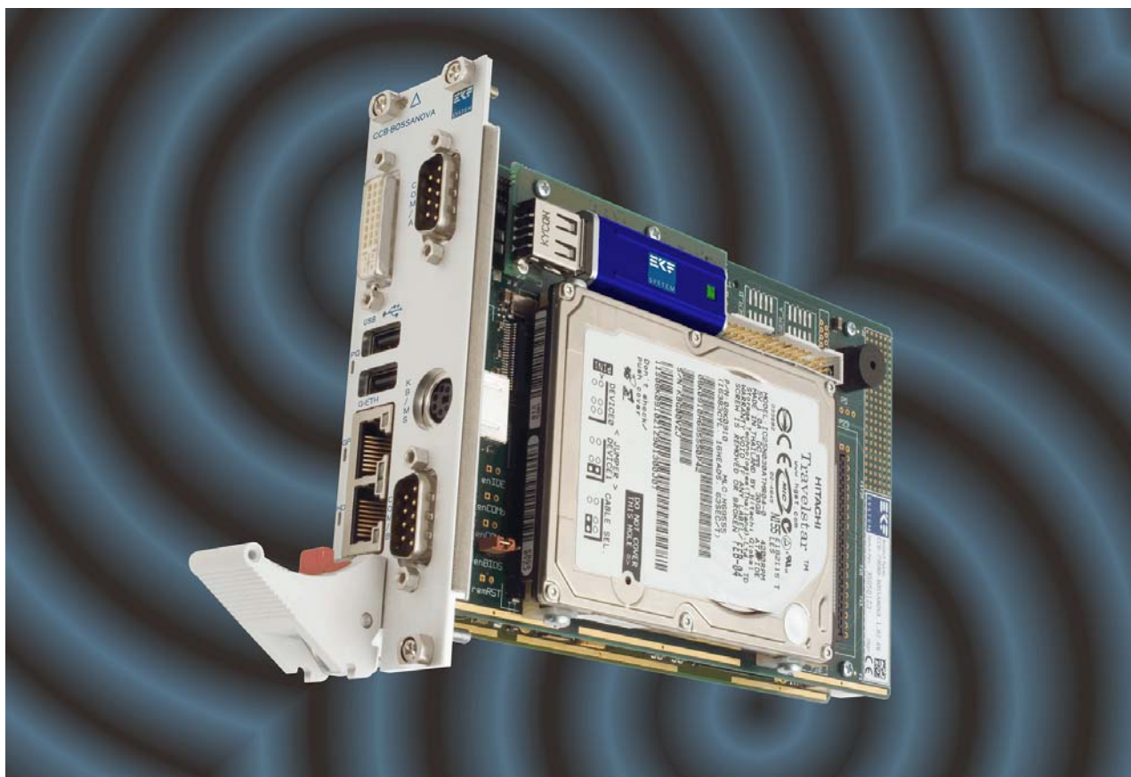
CCD-CALYPSO w. CCB-BOSSANOVA Mezzanine Companion Board & 2.5-Inch HD
