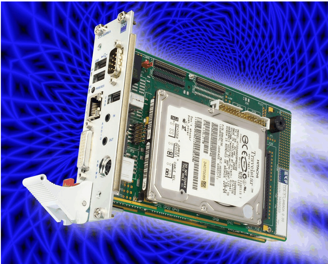
CCA-LAMBADA mounted on top of the CC9-SAMBA, with hard disk option
