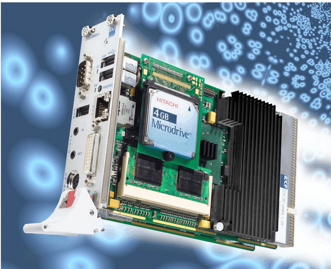
CCA-LAMBADA mounted on bottom of the CC9-SAMBA
