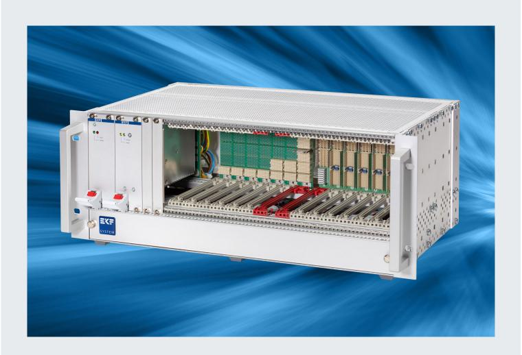
The SRS-8442-SERIAL rack is equipped with two backplanes, left for CompactPCI® Serial cards, right for CompactPCI® Express boards (aka PXI Express™). In order to combine both worlds, a CompactPCI® Serial CPU with a mezzanine bus coupler bridge fits into both system slots, as a 10HP assembly.
