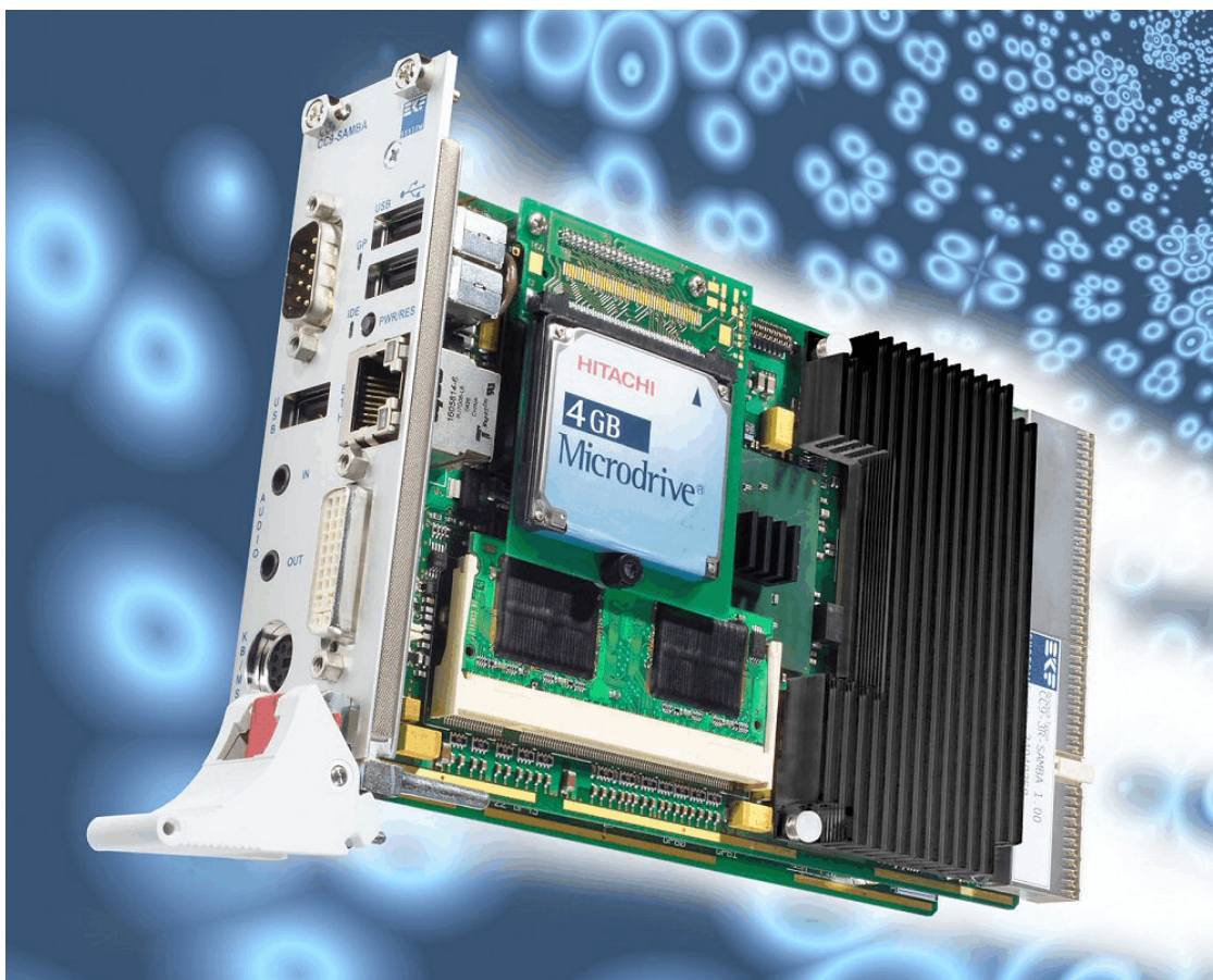
CCA-LAMBADA mounted on bottom of the CC9-SAMBA
