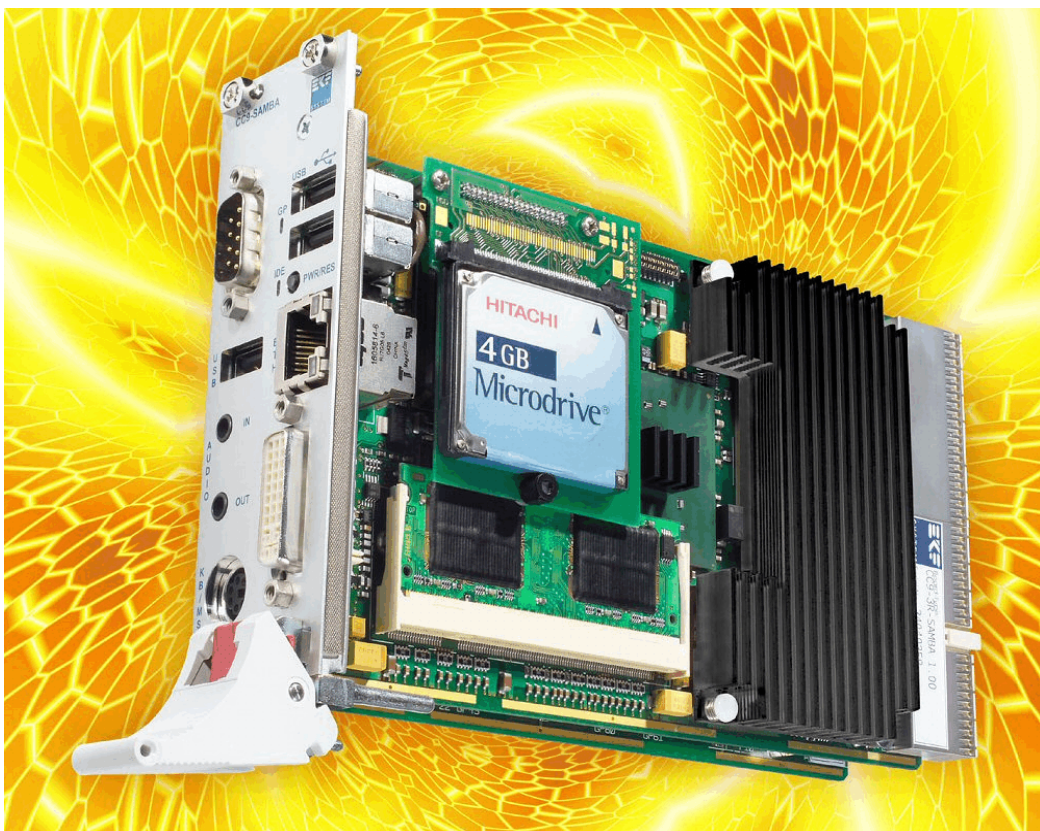
CCA-LAMBADA Mounted on Bottom of the CPU Card
